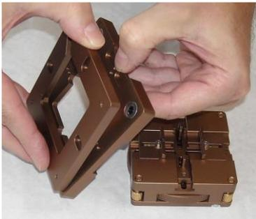
The frame parts **a** and **b** are connected to each other by magnets and can be separated without additional tools.
