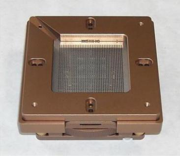
If the template holes are not congruent with the pins of the BGA, the template must be shifted accordingly. Then the parts are screwed together.
