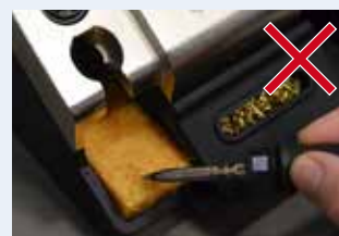
DAMP – NOT WET!
