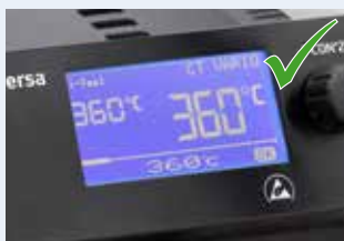
340 – 360 °C for lead-free solder
