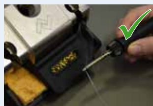
Add new solder after cleaning
