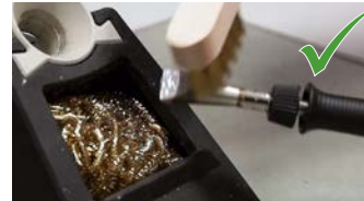
Alternative method: Clean by brass brush (3ZT00051)
