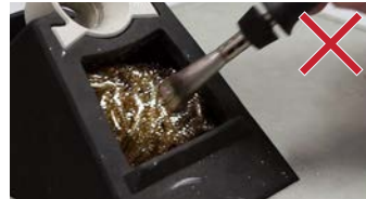
Difficult to clean: Large area and odd shape tips
