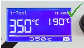
340 – 360 °C for lead-free solder (644 – 680 °F)
