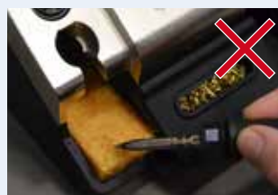
DAMP – NOT WET!
