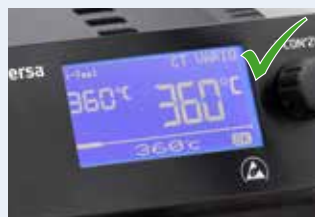
340 – 360 °C for lead-free solder
