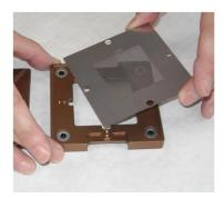
Both an 80x80mm and a 90x90mm stencil can be inserted into this frame.
