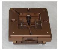
The rebaling station consists of a total of three parts. The parts  $\bf a$  and  $\bf b$  form the two-part frame for the templates. It 80x80mm as well as 90x90mm stencils fit into it. Part  $\bf c$  is the component holder.
