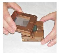
Place the frame with template on the component holder.
