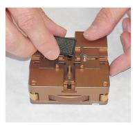
Insert the BGA into the continuously adjustable component holder. The minimum component size is 4x4mm. The maximum component size is 45x45mm.
