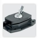
Suitable for all workbenches and tables. Place dimensions  $150 \times 106$  mm. The holder can be screwed on with four through holes ( $\emptyset$  9 mm). A drilling drawing can be downloaded from the website. A small lever pressure is sufficient to fix the ball steplessly and in any practical working position.
