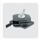
The holder can be screwed to the workbench through 4 through holes (space dimensions  $152 \times 151$  mm), or it can be fixed to steel surfaces with 4 magnets. The 4 high-performance magnets with protective caps have a holding force of 32 kg horizontally and 15 kg vertically (magnets without caps). The magnets are firmly connected to the housing with screws. A drilling drawing can be downloaded from the website.
