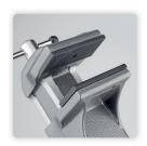
For workbenches or tabletops with a maximum table thickness of 80 mm. The small vice with ball joint can be quickly and easily connect to any table tops thanks to its smooth-running table clamp. A little pressure of the lever is enough and that the clamped workpiece can be fixed steplessly and in any practical working position. He had stable 50 mm ribbed plastic jaws (waffle pattern).
